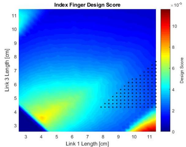
Fig. 2. Optimization results for the linkage connecting to the index finger for  $A=5$ . Dots represent kinematically valid combinations of  $L_1$  and  $L_3$  for  $L_2=8.9$ cm. Set  $L_1 \geq 4.4$ cm due to minimum axes size.
